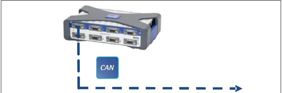
Fig. 7.9 Output to CAN bus (MX840A, connection 1)
